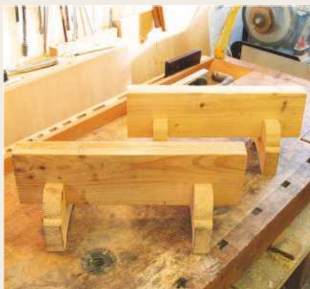
A close up of the little saw horses that I use to raise up work to a comfortable height on the bench. You can easily make them up from offcuts; they don't have to have shaped legs!
